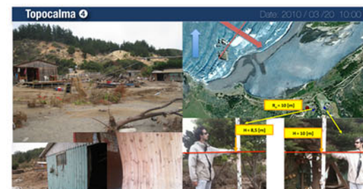
Topocalma is located a few kilometers north from Pichilemu. Here locals reported the wave approaching directly into the beach. Run up levels showed a significant increase with respect to communities located further south, reaching up to 10 m locally.
