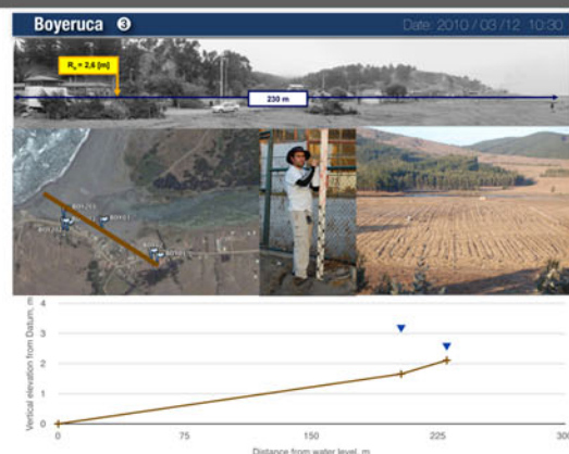
The coastal configuration of Boyeruca is typical of central Chile, where the interaction between a stream and waves tends to form bars and dunes at the discharge. These were completely reconfigured due to the tsunami, which propagated several kilometers inland as shown by boats found in crop fields. The most destructive waves were reported to be of bore-like nature approaching from the north.
