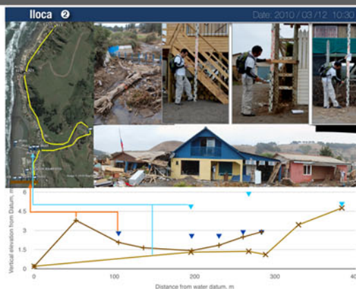
Iloca sustained widespread damage, although the maximum run up was about 4.7 m. Debris floating bodies caused damage to the small dam used for the town's water supply, located a few kilometers inland along the Iloca river. Although some of the residential areas were protected by a coastal dune, the tsunami entered from the back side of the dune. Despite the damage, no casualties were reported here due to the appropriate community response and training.
